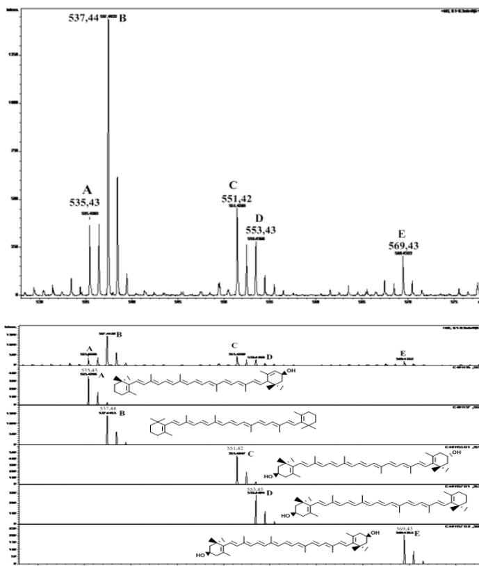
**Figure 1:** Liquid Chromatography – Mass Spectrometry and MS/MS spectra of OFSP flour extract
