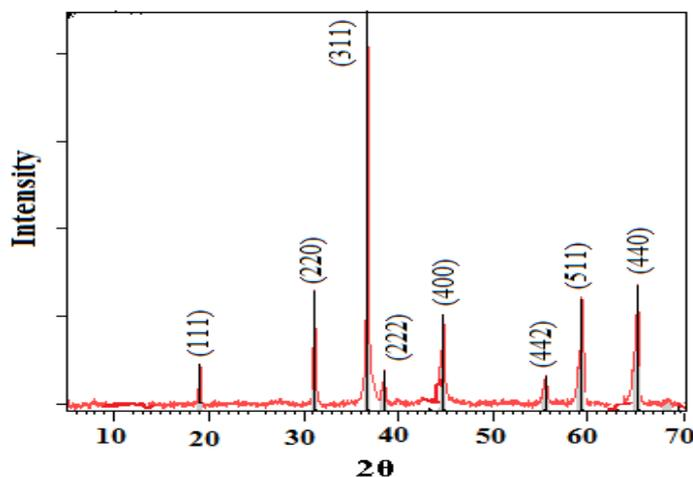
**Figure 1.** X-ray diffractogram of  $Ni_{0.9}Co_{2.1}O_4$  prepared at 350° by sol-gel method (propionic acid)
