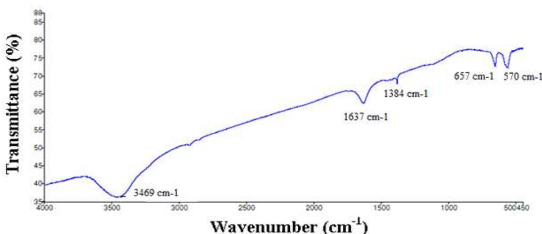
**Figure 2:** FTIR spectrum of Ni<sub>0.9</sub>Co<sub>2.1</sub>O<sub>4</sub> prepared at 350° by sol-gel method (propionic acid)
