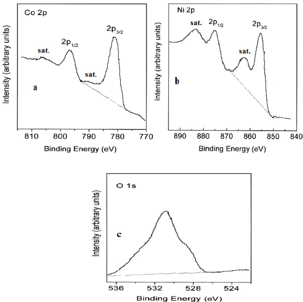
**Figure 3** :XPS spectra of  $\text{Ni}_{0.9}\text{Co}_{2.1}\text{O}_4$ : (a).  $\text{Co}_{2p}$ , (b).  $\text{Ni}_{2p}$  and (c).  $\text{O}_{1s}$
